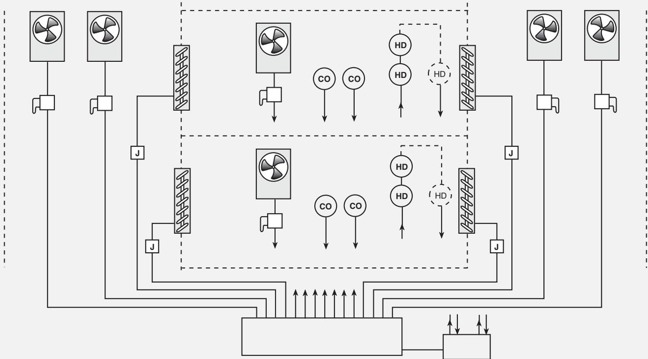
Colt can provide a full system comprising control panels, carbon monoxide (CO) detection, and an addressable heat/smoke detection system. Alternatively our control panels can be linked to the building's fire alarm system..
